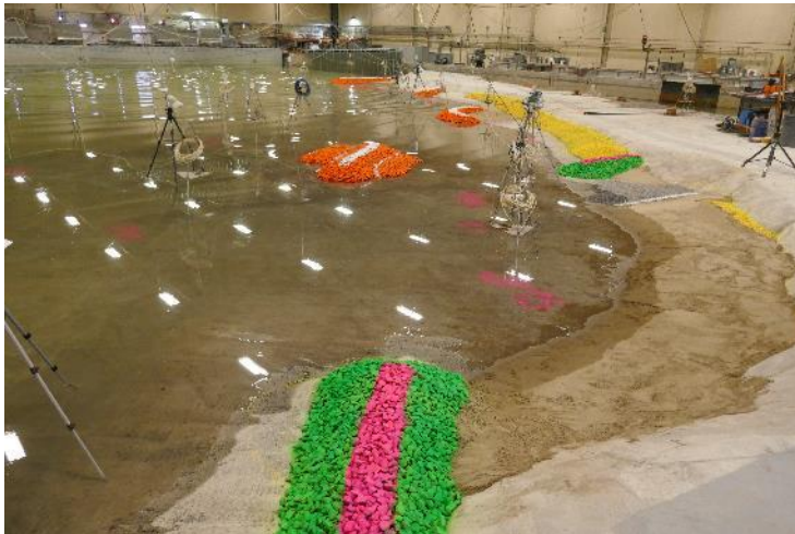
Figure 3. Three-dimensional 1:20 scale physical model of the northern BC site’s shore protection scheme at NRC-OCRE’s Large Area Basin in Ottawa.
